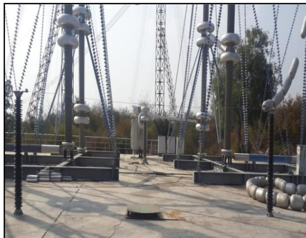
Figure 4: Schematic view of unipolar DC line experimental line setup.
